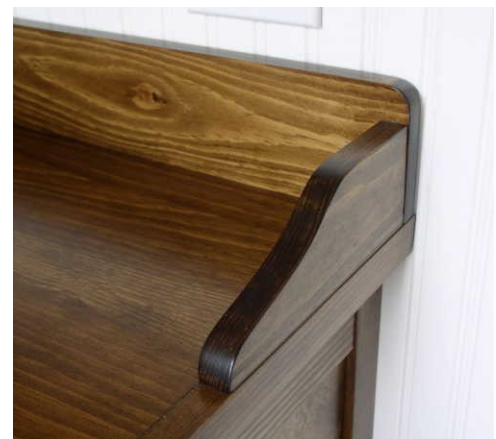
Fig. 26 - 3" h side splash profile was drawn freehand on paper template
