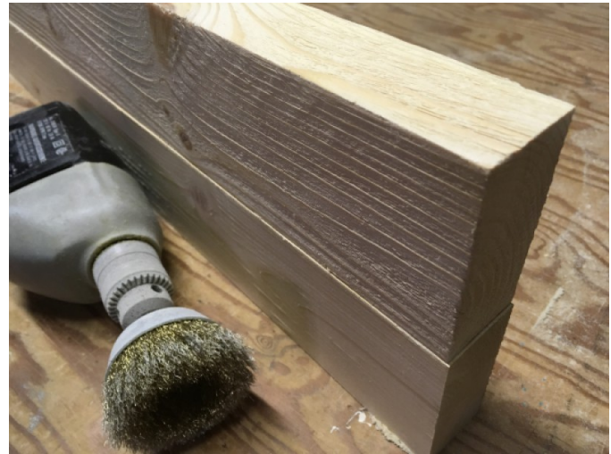
Fig. 2: The top piece shows the effect of the wire brush treatment compared to the original on the bottom.
