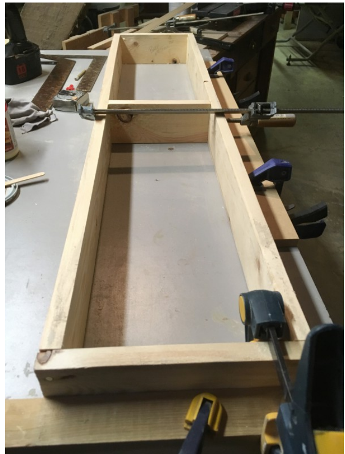
Fig. 3: Clamp Cleats to the work bench to help hold the parts while nailing.
