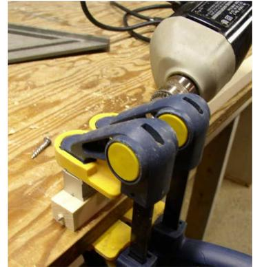
*Fig. 15 – Exit hole should be centred on end grain*
