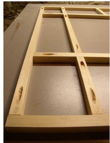
*Fig. 16 - Back of a similar 13/16" face frame with pocket holes - ready for assembly*
