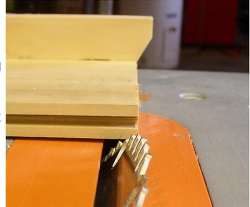
*Fig. 6 To cut the end bevels, line up the top edge with the mitre on the mitre gauge fence.*
