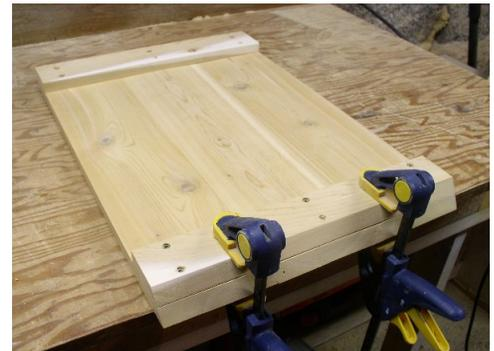
**Fig. 8** Bottom cleats are attached to boards with 1 1/4" deck screws.
